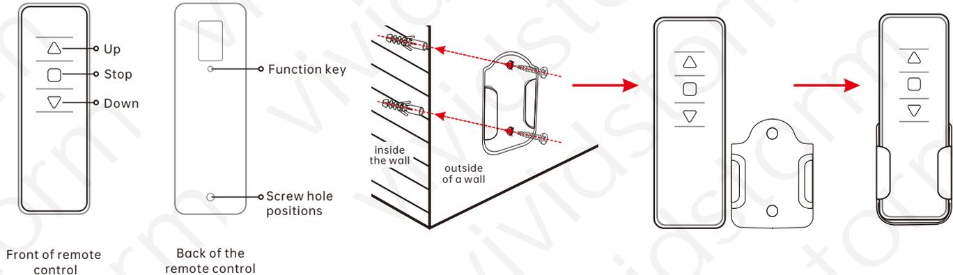
When the battery of the remote control needs to be replaced, as shown in the figure below, unscrew the cover of the remote control with a small screw, then replace the new button battery, close the cover of the remote control, and tighten the screw to prevent the loose battery from falling off;
