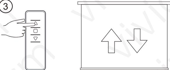
Lower the screen to the desired height. Press the 'Up' key or 'Down' key for fine adjustments based on the height requirements. For significant adjustments, press and hold the 'Up' key or 'Down' key for 2 seconds to continuously adjust the screen position.
