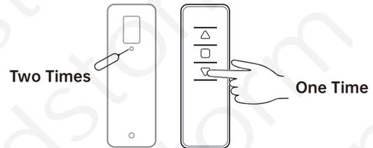
After confirming the height, use a pointed tool to press the 'Function' key on the back of the remote control 2 times. Within 10 seconds, press the 'Down' key on the remote control 1 time. The lower axis of the screen will jitter once, indicating the successful lower limit setting. Fully close and then reopen the screen to ensure the correct screen height.
