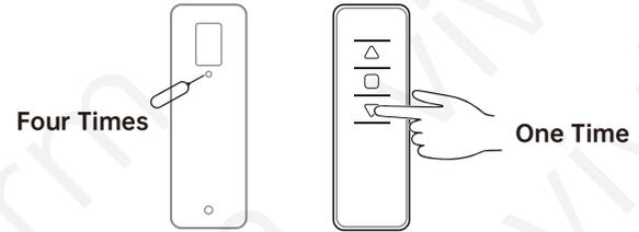
Enter adjustment mode: Use a pointed tool to press the 'Function' key on the back of the remote control 4 times, then within 10 seconds, press the 'Down' key on the remote control 1 time. At this point, if the lower axis of the screen jitters once, it indicates entry into the limit adjustment state.
