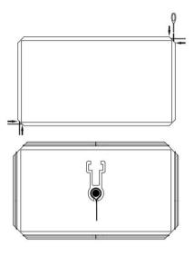
10. The pair lift the inner frame horizontally and put it on the screen base fabric, adjust the position of the inner frame to make it centered.
