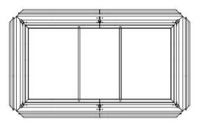
11.Insert the T-nuts into the corresponding positions of the tie rods respectively, and pay attention to distinguishing directions
