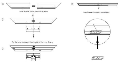
Align the outer frame middle support joint with the inner frame splice joints threaded holes.
