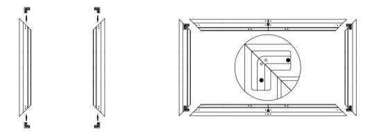
3. Align outer frame four-corner support joint with the threaded holes of Elbow Joints (inner frame) and fix the two screws in the middle of the Elbow Joints (inner frame) with (M4\*6) screws.
