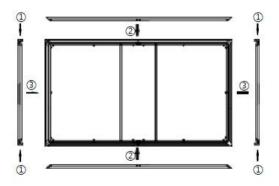
16.Remove the release film on the side A of the Velcro, and paste the three pieces of Velcro on the area shown in the Image.
